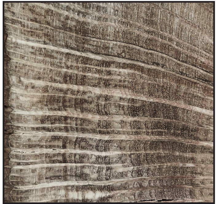
Oak Rings 1. Narrow vs wide rings indicating growth rate. Photo by Ron Ruppert.
